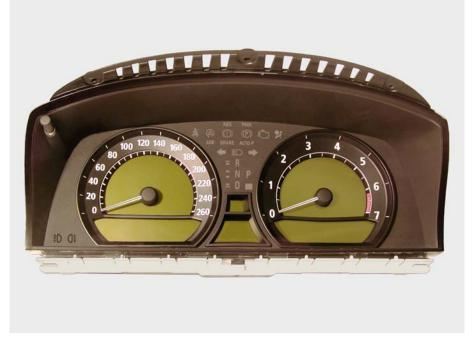
The fuel and temperature gauges have been deleted from the instrument cluster and are now an On-Board Computer and Check Control display respectively.
